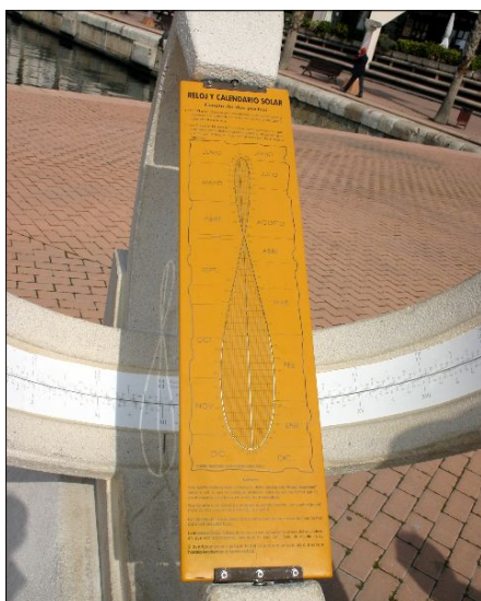
Fig. 2. A closer view of the gnomon panel showing the complete analemma and its bright outline on the dial.
