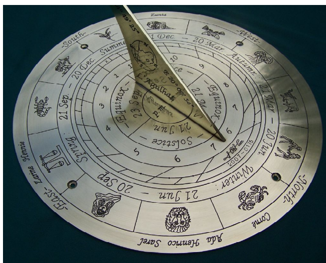
Fig. 2. The most southerly dial in South Africa, at the Cape of Agulhas. Note anticlockwise, longitude-corrected, hour numerals!
