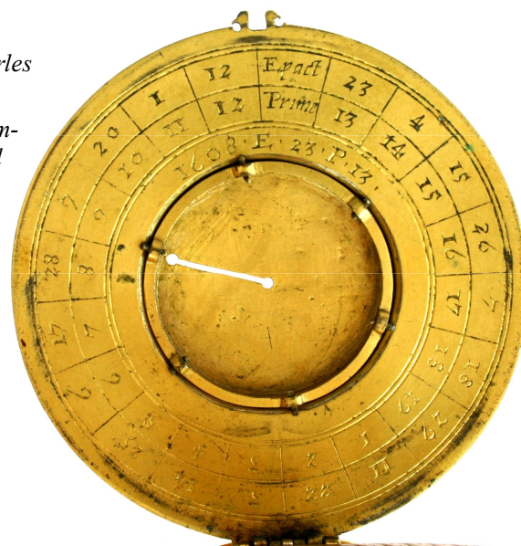
Fig. 6. A tide computer on the underside of the Whitwell compendium.
