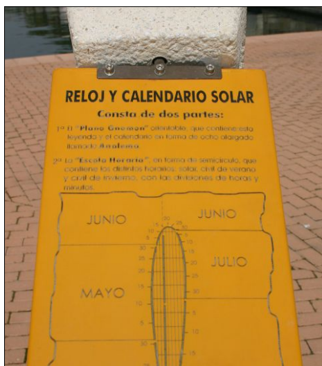
Fig. 3. The top of the gnomon panel with the date marked every 5 days: the horizontal lines are spaced vertically to show the changing declination of the sun every 1° whereas the vertical lines are separated by one minute in time thus giving the equation of time. The date can be interpolated by masking the slot until the cut-off point is found on the time scale.
