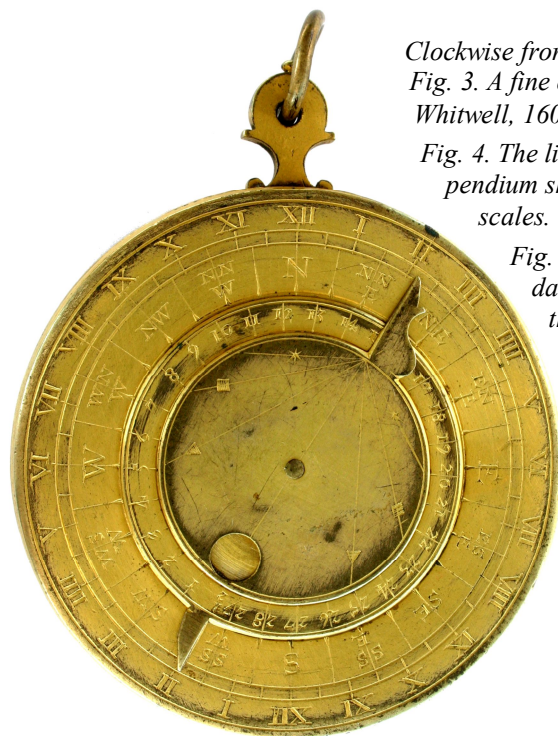
Fig. 6. A tide computer on the underside of the Whitwell compendium.
