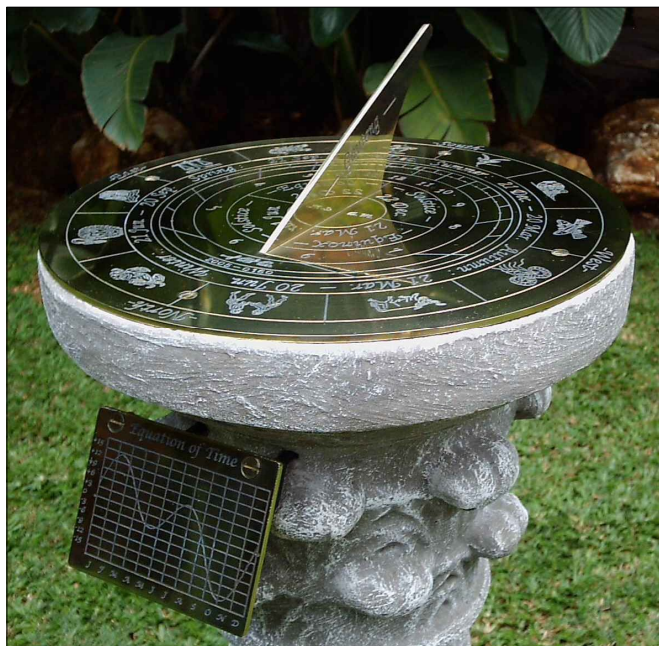
Fig. 3. An installed dial, with EoT plaque.
