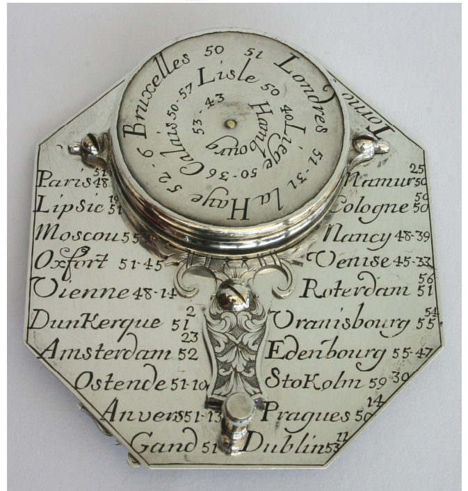
Figs. 15 & 16. Butterfield dial by 'P le Maire A Paris, A la Pierre d'Aiman', the underside showing his unusual list of northern towns.
